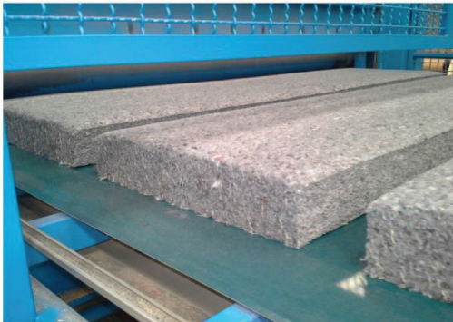
Recycled textile insulation being manufactured
