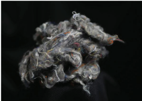
Close-up of textile insulation
